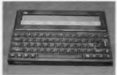
The Cambridge Z88 uses a 3 MHz Z80-compatible processor and a full sized rubber keyboard – RAM can total up to 1.568 megabytes!.
