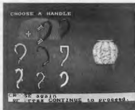
Figure 1. Design a teapot: after selecting a suitable pot body, you are given a choice of handles. The images were digitized using DigiView, then cleaned up with Deluxe Paint on an Amiga 500.
